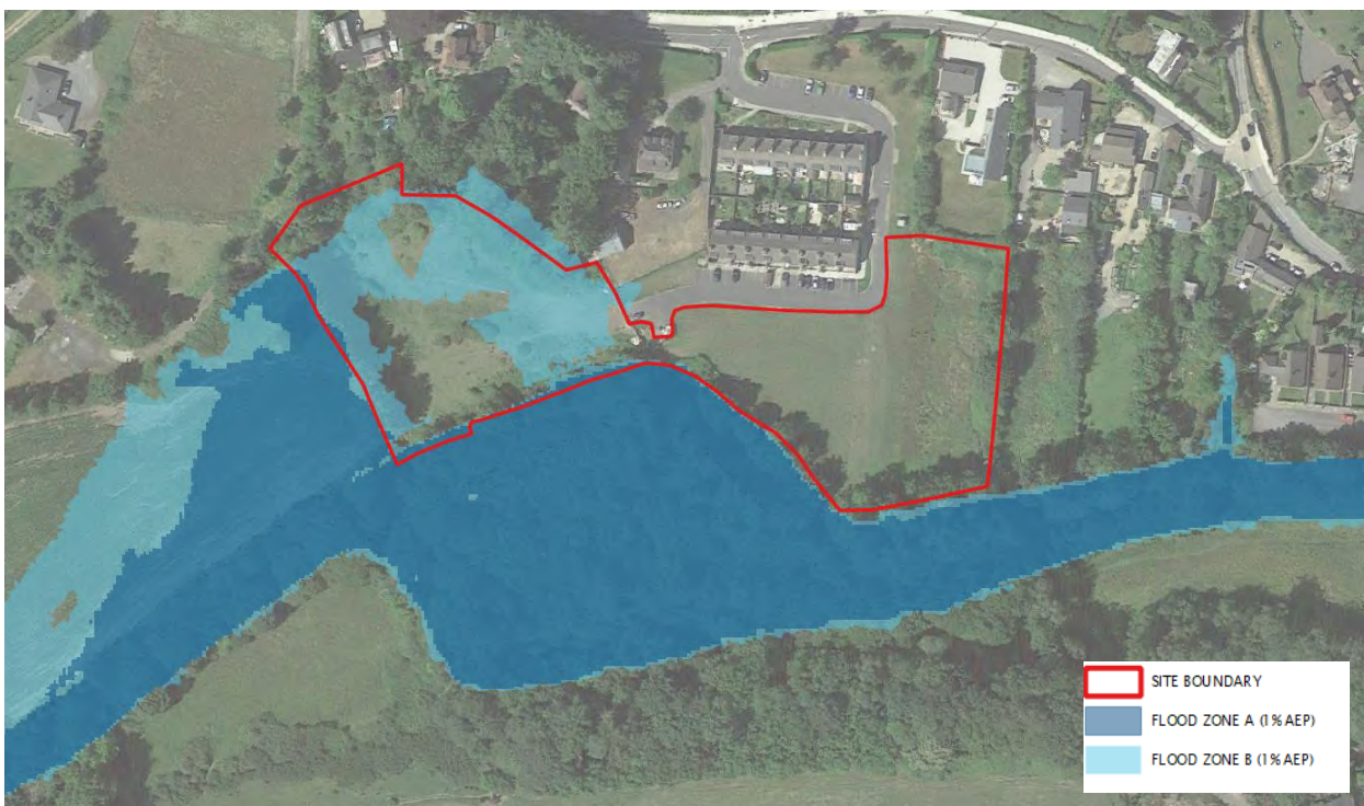
Figure 5–1: Flood Zone A and B
