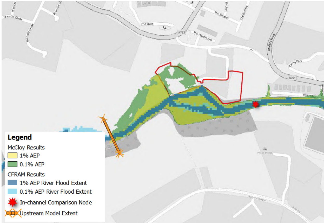
Figure 5–2: Comparison of modelled results with CFRAMs
